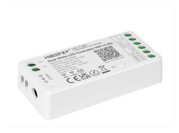
LED Controller CCT 12-24VDC 12A Milight FUT035W WiFi is a small device used to control LED CCT lighting. It allows you to change the light intensity and color temperature of the connected CCT LED strip, Control via a remote control or smartphone application. Support push button to turn on/off the light, and change the light intensity. The controllers acts as a repeater, while maintaining a 30m spacing between successive elements, allows for unlimited range.
