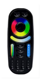
An advanced remote control designed for MONO/CCT/RGB/RGBW/RGB+CCT light sources, allows you to control four zones, in each zone can work with many controllers at once. Using it you be able to smoothly adjust the brightness, color of light, and the color temperature of white light.
