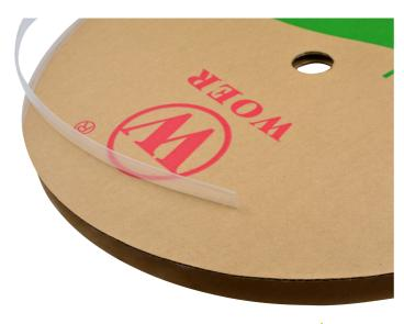
Temperature ranges : -55°C $\sim$ 125°C Use under acid and alkali. Easy for use, using oven or heating gun and it will shrink, shrinking temperature start at 70°C and shrunk totally at 125°C, suggest the shrink-time had 3 minutes.
